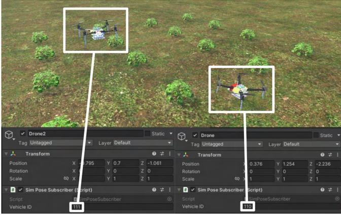
Fig. 3. Unity setup for multiagent simulation. Users only need to make replicates of the drone object and specify different vehicle IDs in the Inspector window.
